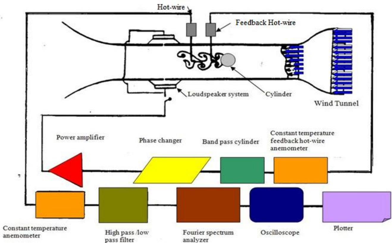
Figure 3. Top view of experimental setup and feedback control loop
