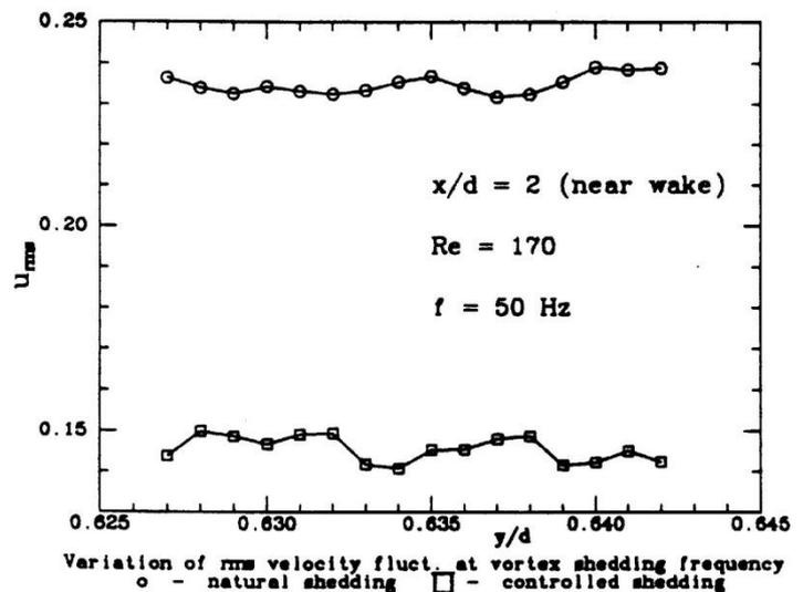
Figure 4: Longitudinal velocity fluctuations versus vertical locations.
