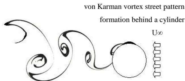
**Figure 2.** The vortex shedding rolled from upper shoulder of a stationary circular cylinder.
